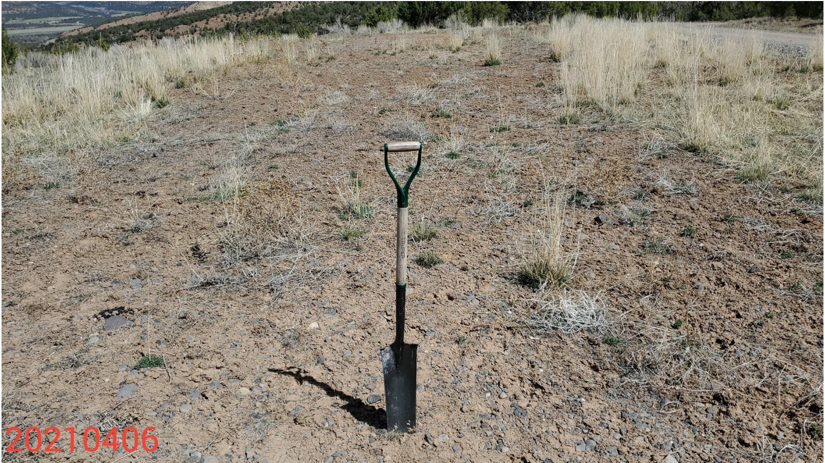
Photo 5: Photo shows large areas of the Location remain bare and graveled. Photo shows example of a compaction test pit performed on the Location; compaction concerns evident at surface of the Location; unable to easily penetrate soil surface.
