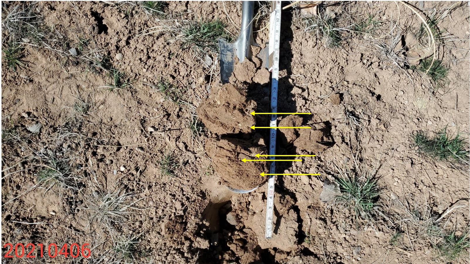
Photo 9: Photo shows another example of a compaction test pit performed on the Location. Photo shows “platy” soil structures observed within the first 4-6 inches of the soil. These structures are thin, flat plates of soil that lie horizontally and are usually found in compacted soils; unable to find evidence that sufficient compaction alleviation was performed on the Location in accordance with 1004 Rules
