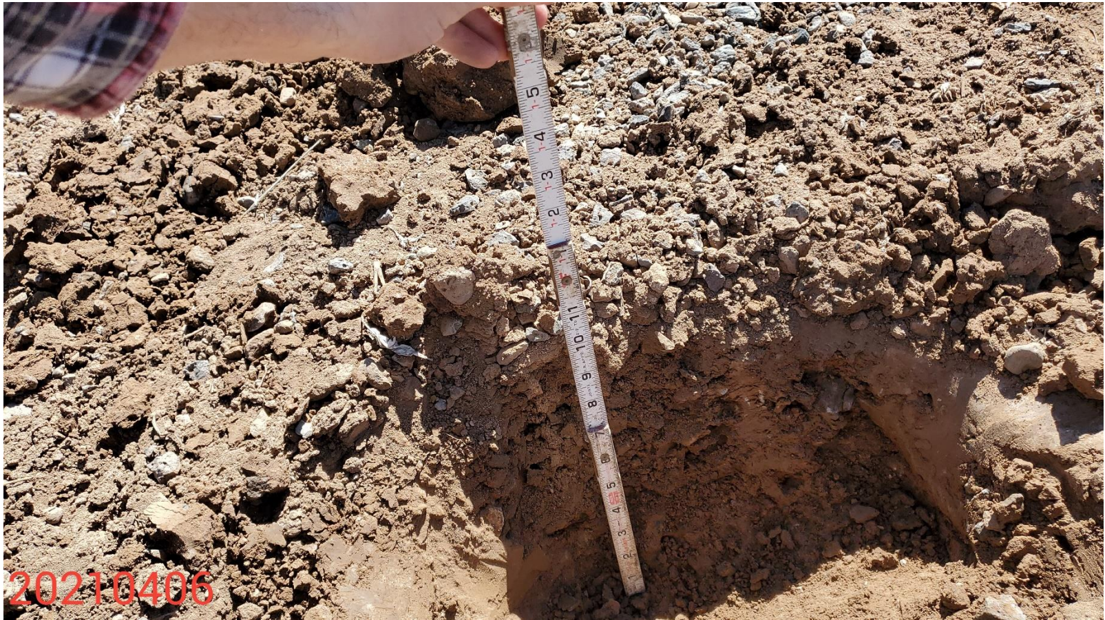
Photo 8: Photo shows example of a compaction test pit performed on the Location. Zones of compaction observed within the first few inches below soil surface. Gravel also observed to not have been removed.
