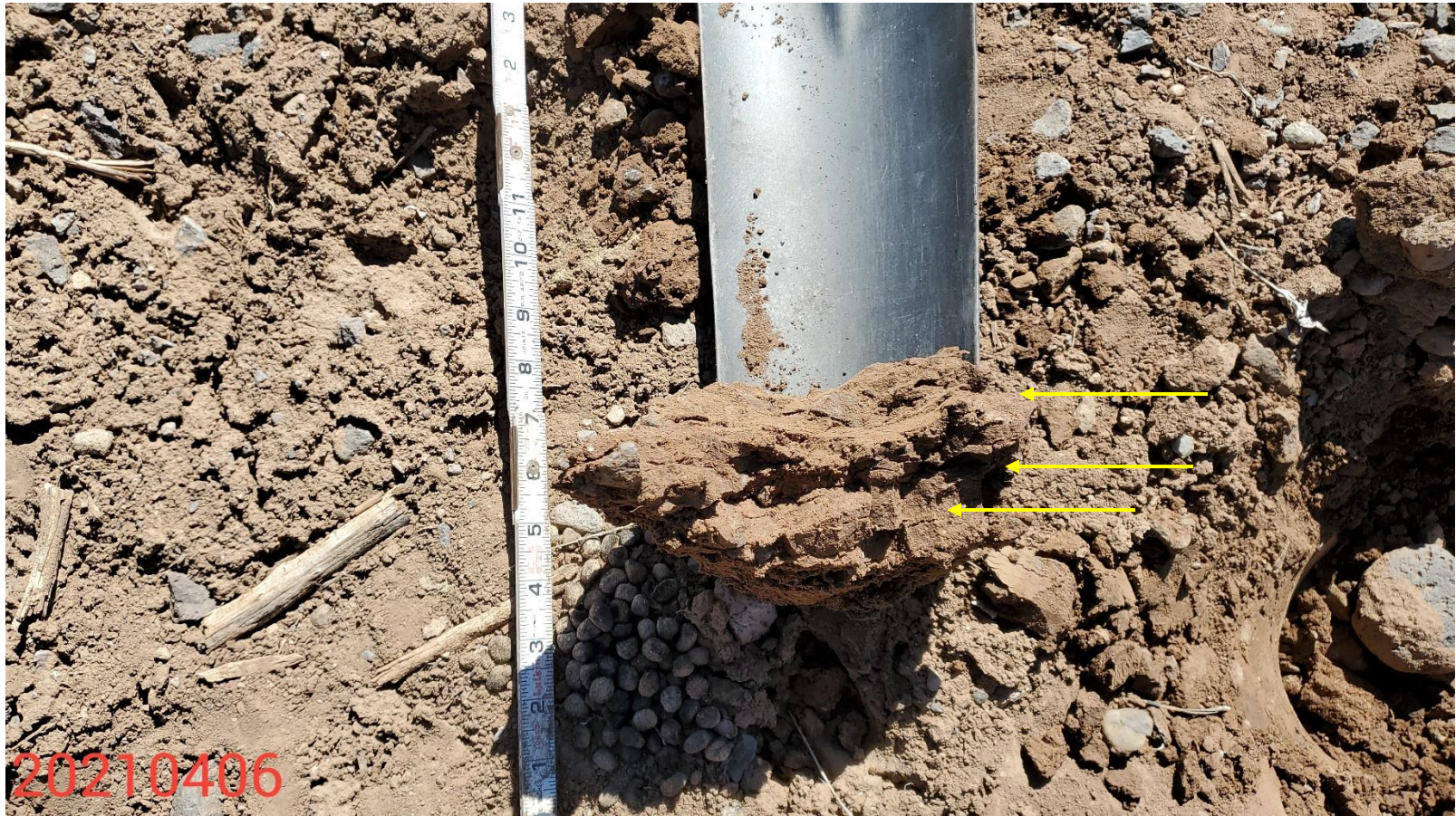
Photo 7: Photo shows example of a compaction test pit performed on the Location. Photo shows “platy” soil structures observed within the first 4-6 inches of the soil. These structures are thin, flat plates of soil that lie horizontally and are usually found in compacted soils; unable to find evidence that sufficient compaction alleviation was performed on the Location in accordance with 1004 Rules
