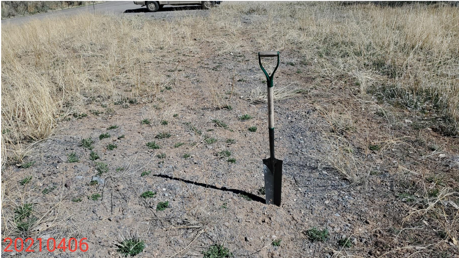
Photo 4: See comments under photo 1. Reclamation Specialist conducted test pits throughout the Location; gravel remaining and compaction remains evident; photo shows example of areas where compaction was evident at the surface; Reclamation Specialist unable to easily penetrate soil surface.
