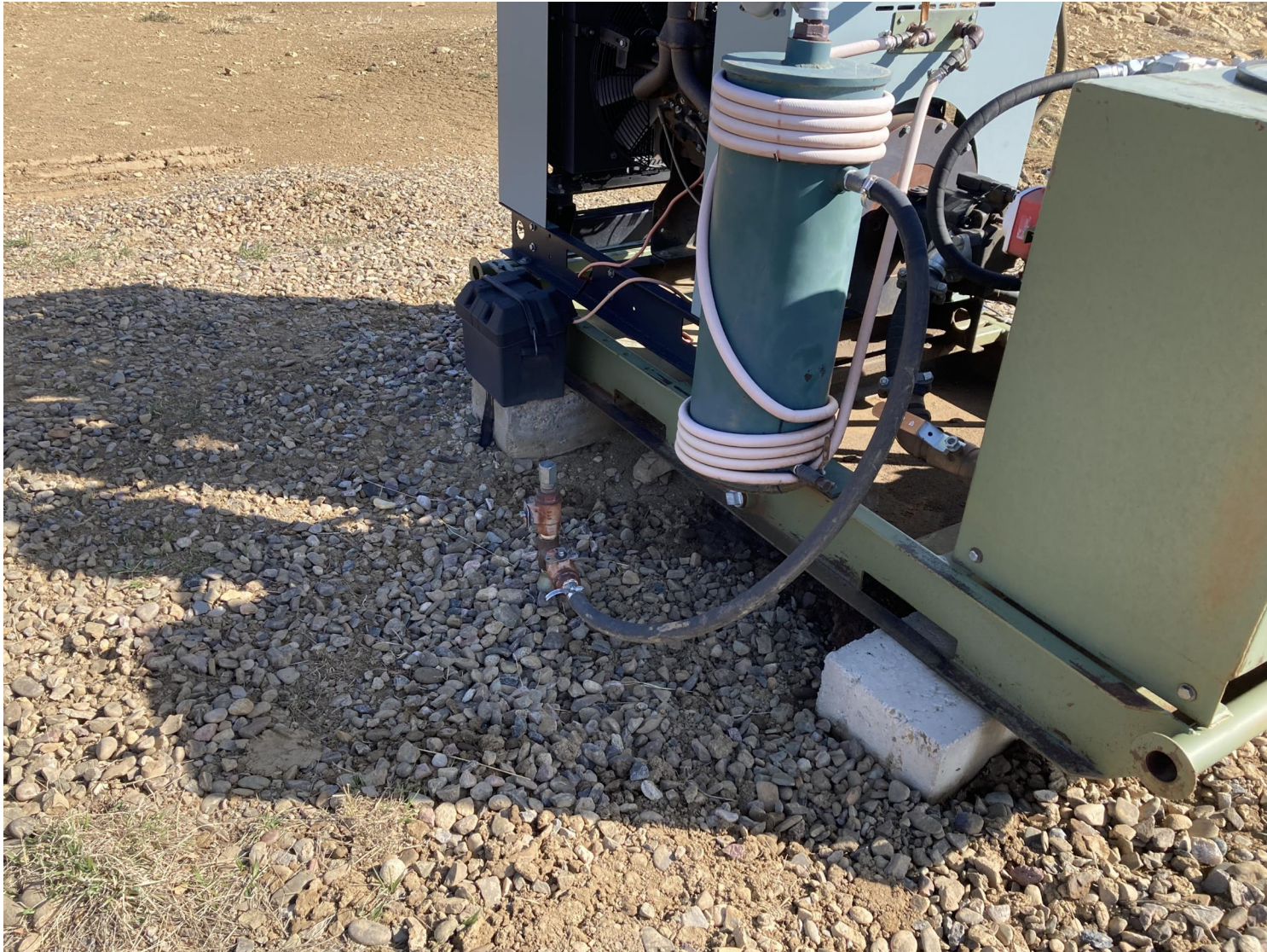
PHOTO 2: THE HYDRAULIC LEAK WAS REPAIRED AND THE IMPACTED SOIL WAS REMOVED.
