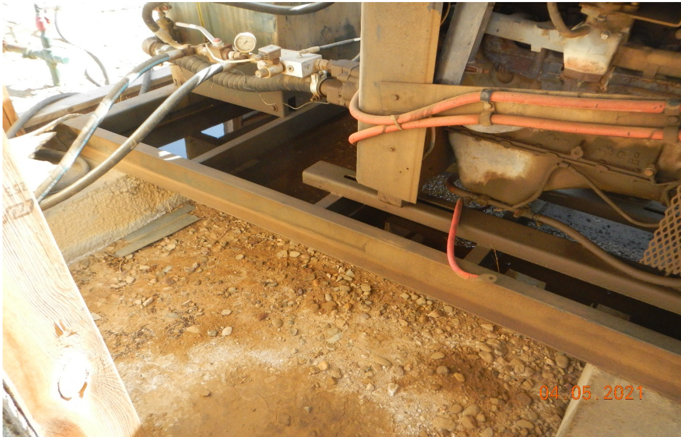
Photo 2. There is oil stained soil near the engine and oil in the engine skid.
