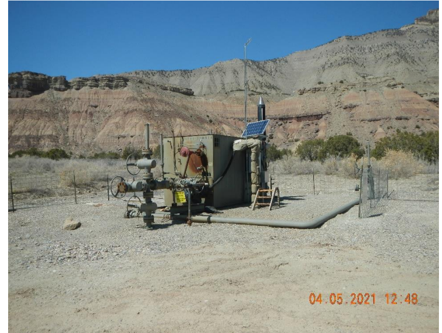
Fencing partially down around separator.
