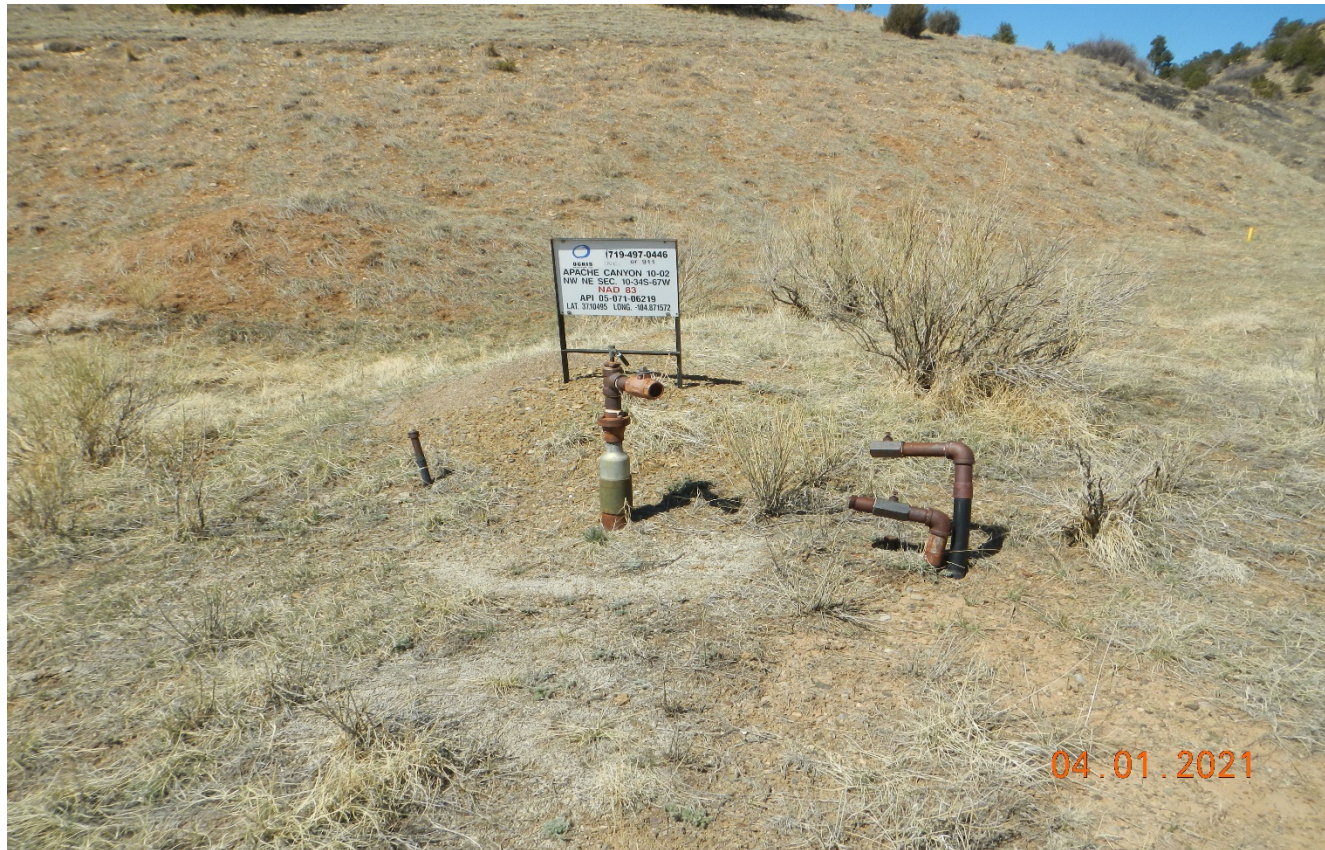
Photo 2. Well is temporarily abandoned. No LOTO on pipe risers.
