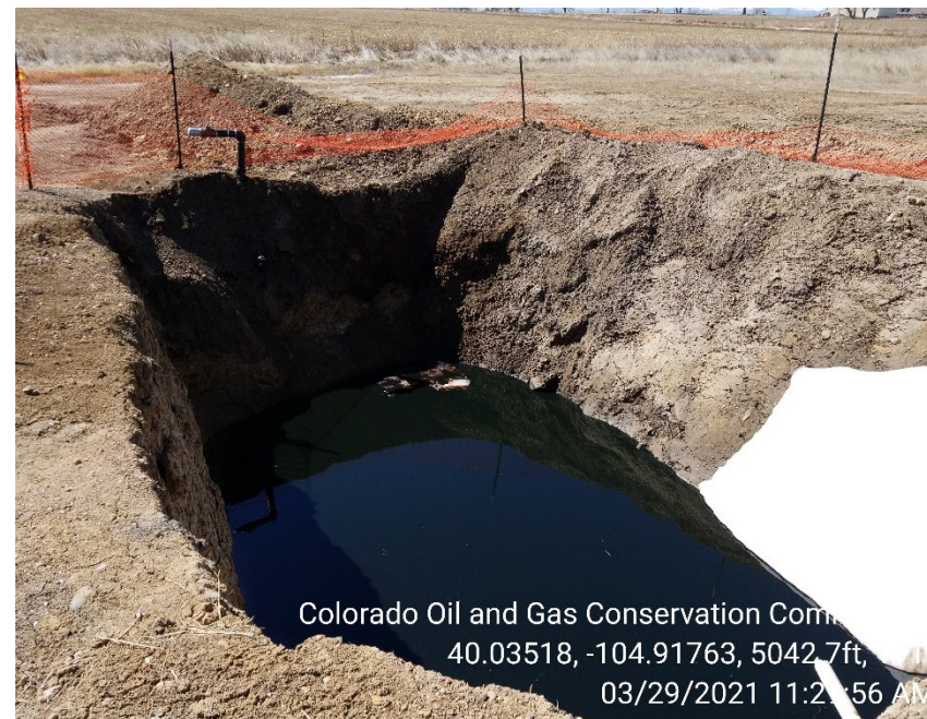
Photo 2 – Free product observed on groundwater in open excavation. Fencing down around open excavation.
