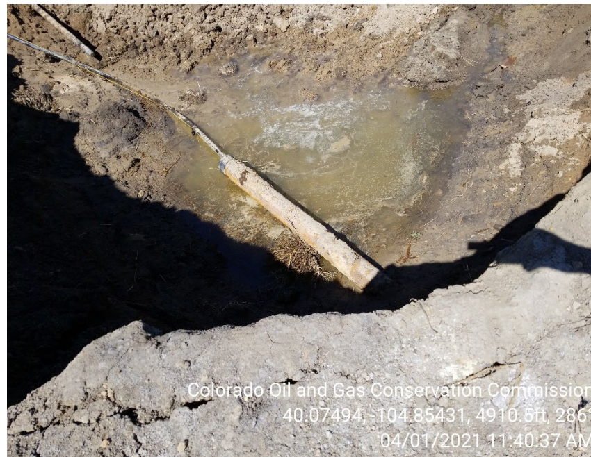
Photo 10 – Groundwater with hydrocarbon sheen observed in open excavation.
