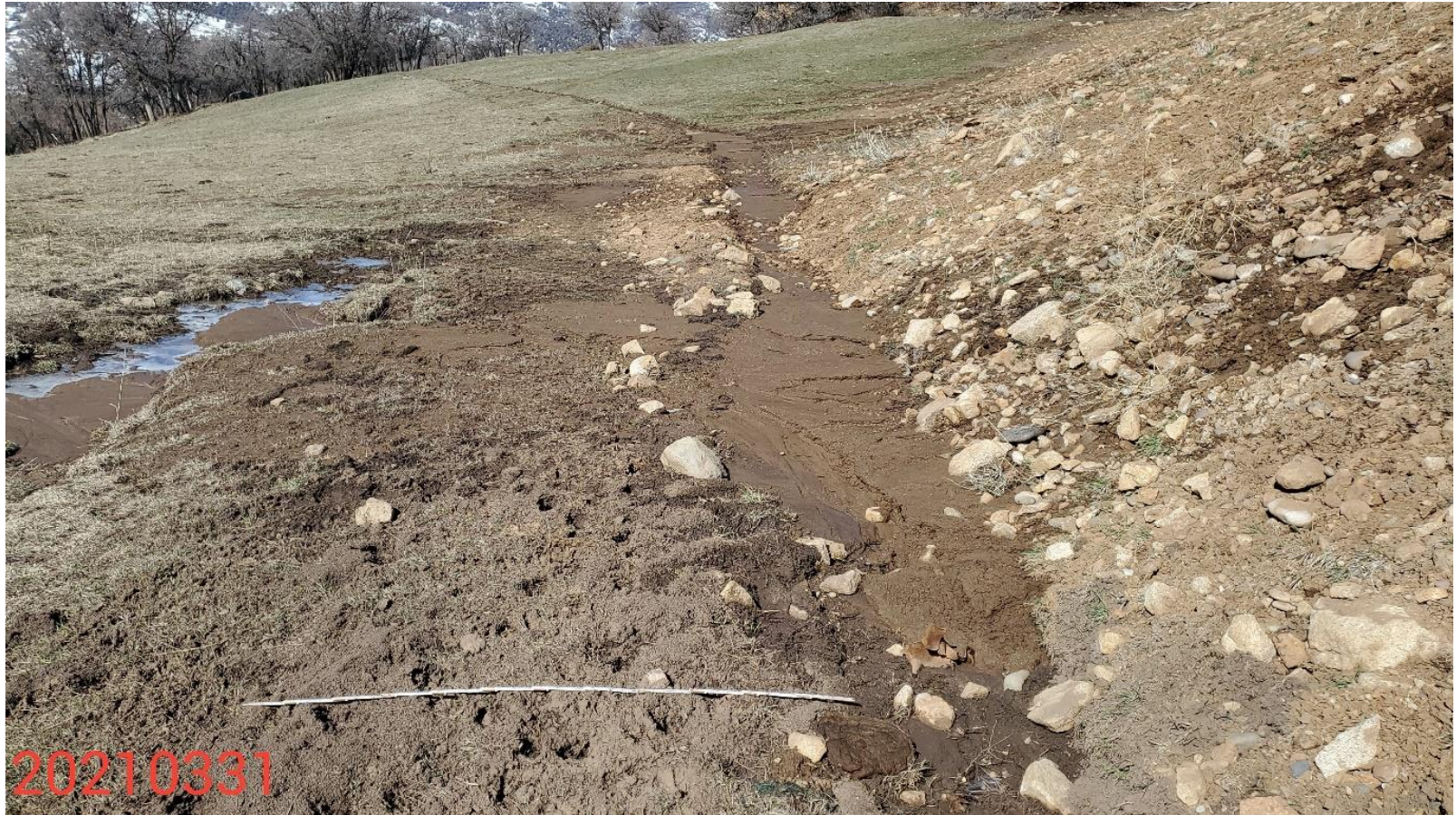
Photo 22: Photo shows off-site sediment discharge on the southwest end of the Location, facing west. 6 foot measuring stick for reference.
