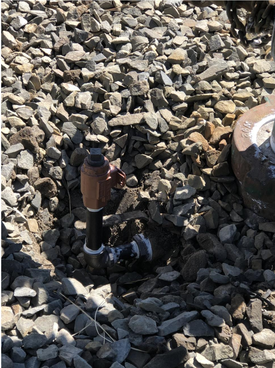
Bradenhead has been plumbed to the surface to comply with Rule 341
