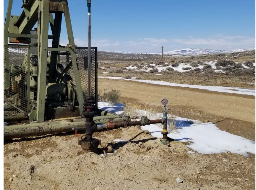
Photo 2. No bradenhead access apparent.
