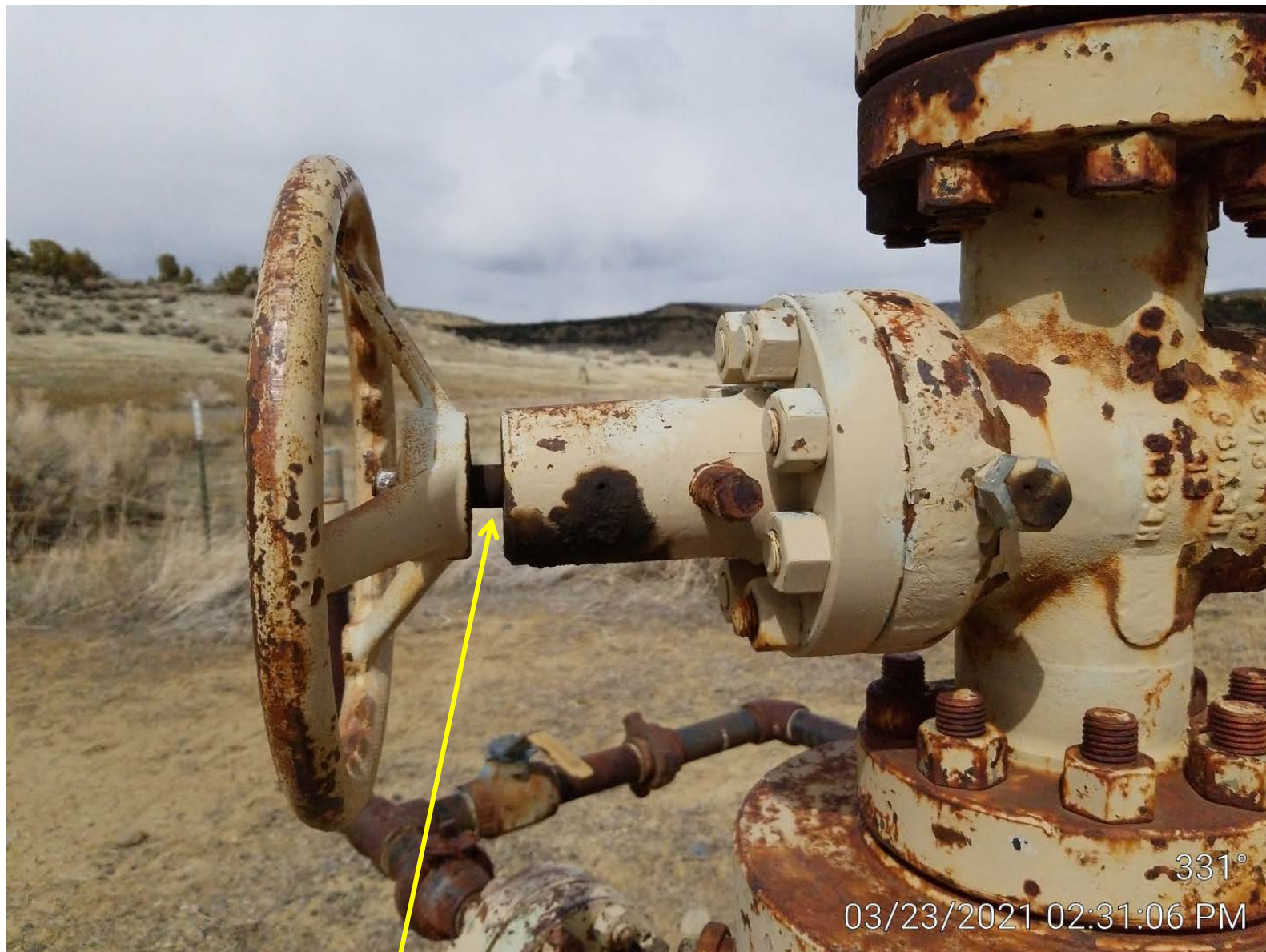
Photo 3. Well gas leak.
