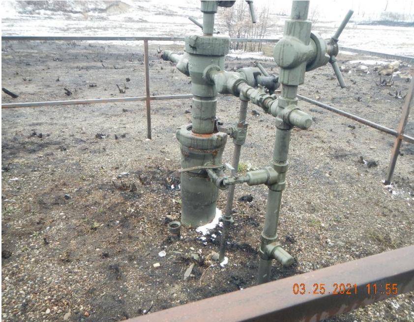
Open ended 2" unused riser at well
