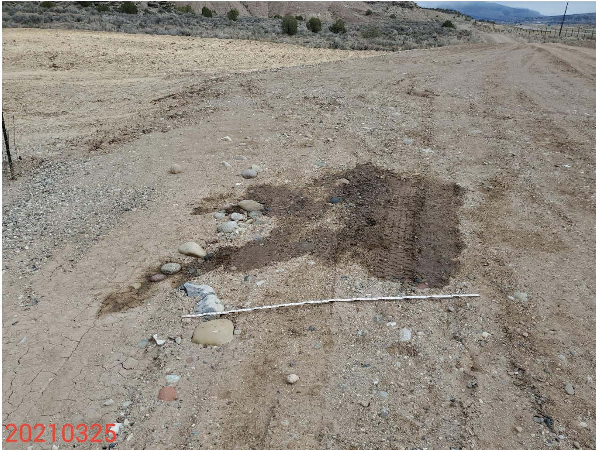
Photo 3: Photo shows stained soils observed next to wells. 6 foot measuring stick for reference.
