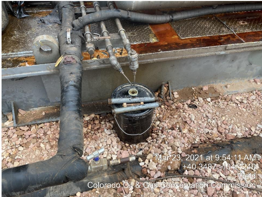
Photo #12 Packing vent lines dripping into bucket
