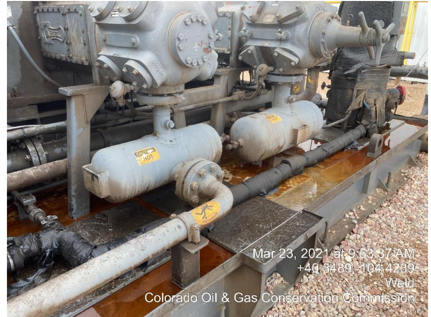
Photo #4 Oily Skid/ Mechanical Conditions
