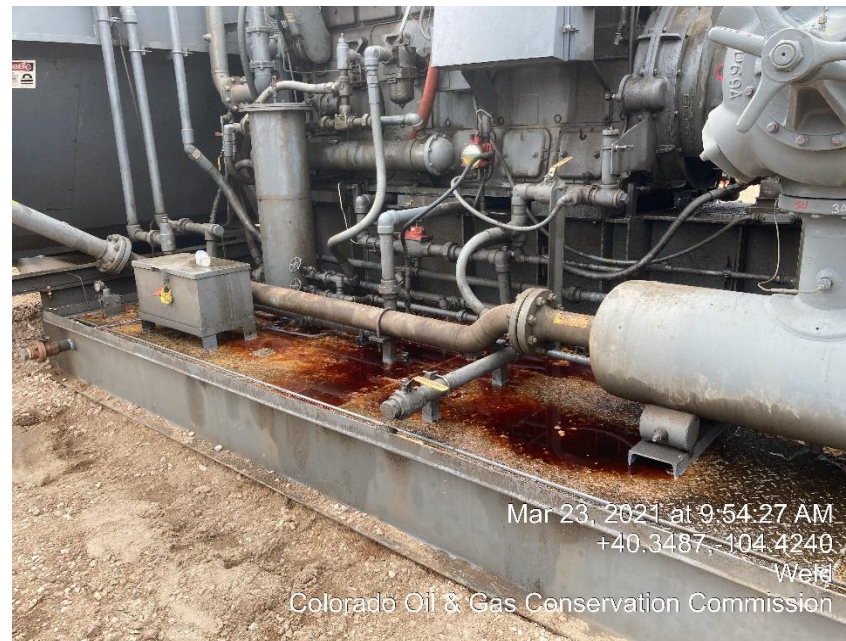
Photo #8 Oily Skid/ Mechanical Conditions
