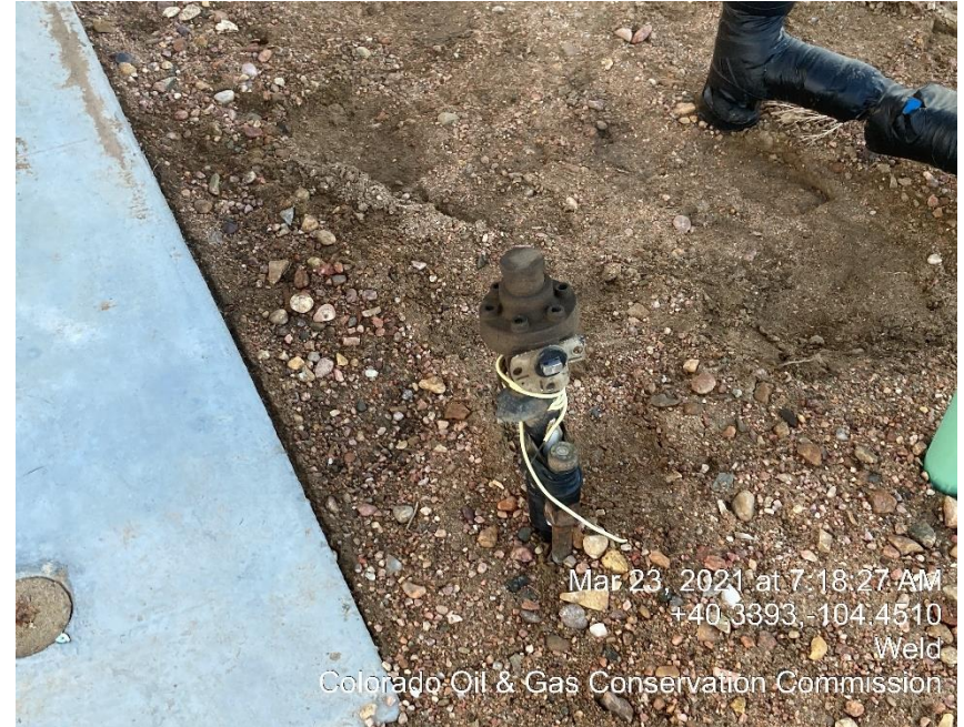
Photo #6 Unmarked Riser
