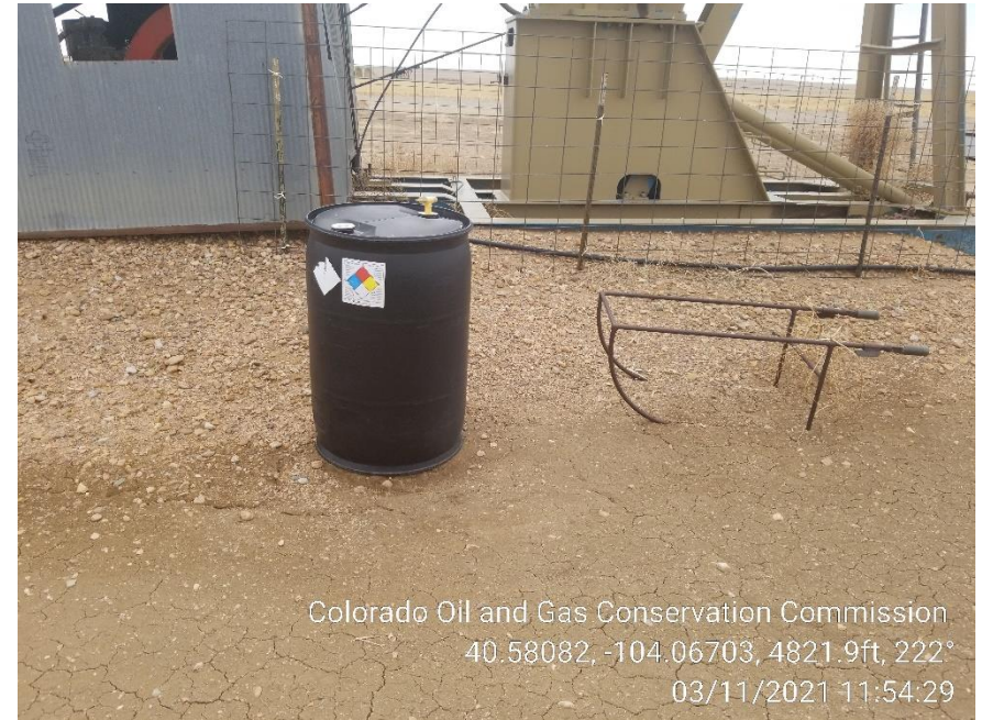
Photo 4 – Black Container – Missing Content and NFPA Label has faded
