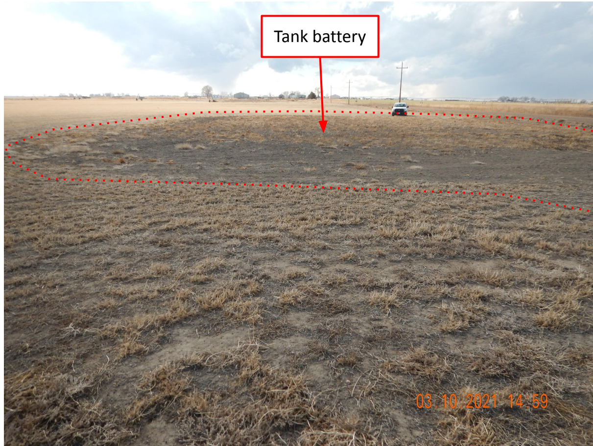
Photo 2. Photo taken east of the tank battery location, facing West. Photo illustrates all equipment has been removed from the tank battery. However, it does not appear the tank battery was properly contoured to the surrounding area and does not have any establishment of alfalfa. If the location is not properly contoured, then flood irrigation is likely compromised and not successfully being irrigated.
