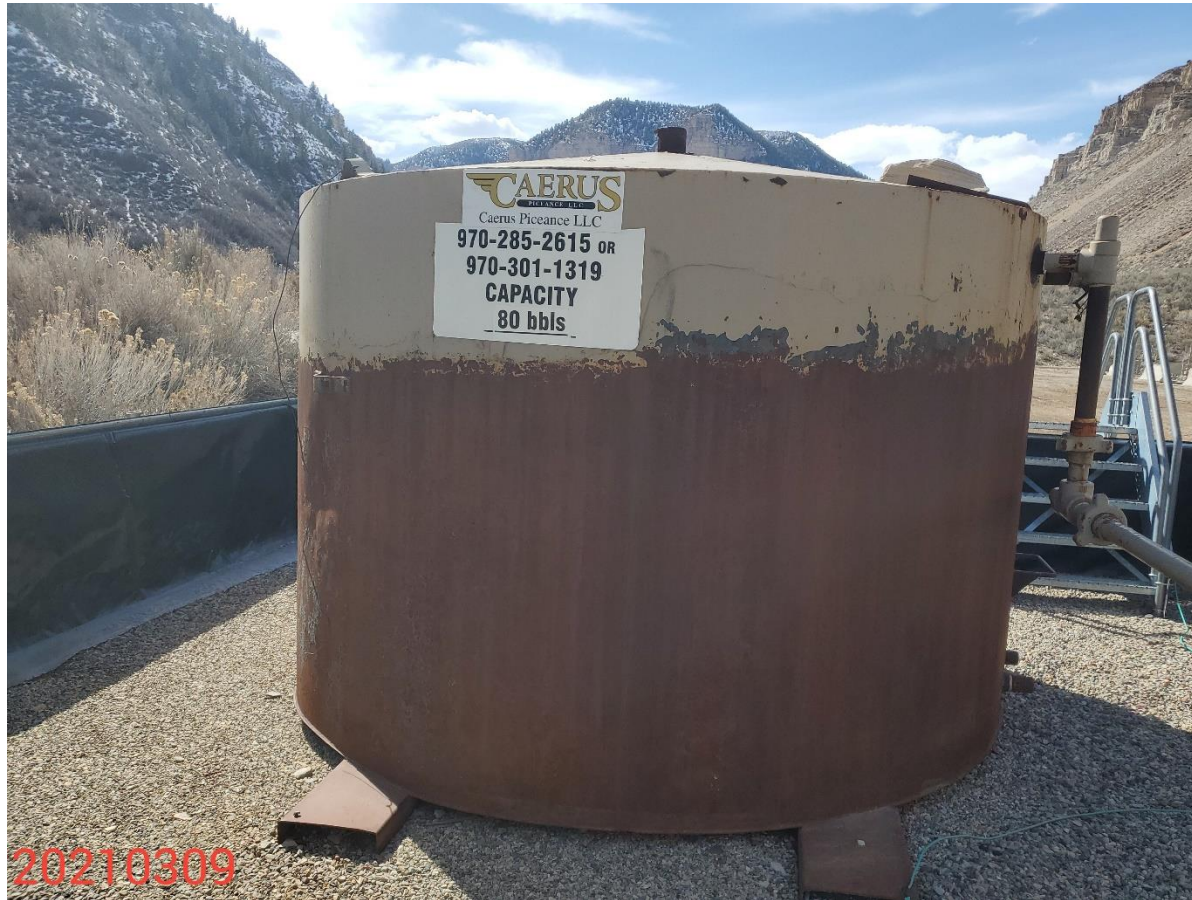
Photo 5: Photo of the 80 bbl produced water tank with emergency contact number.
