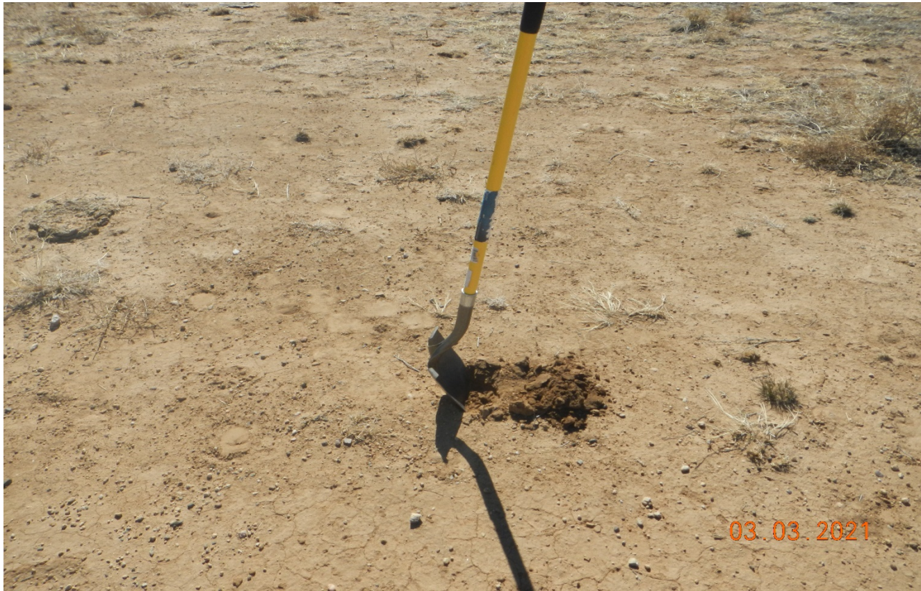
Photo 6. Soils are compacted at the location. Soils need to be decompacted by cross ripping to a depth of 18 inches. Compacted soil are preventing vegetation establishment. The shovel could not penetrate past 2-3 inches.
