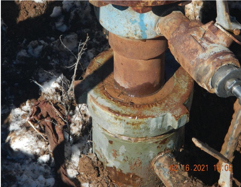
Gas leak observed at the top of the wing nut on the intermediate casing.
