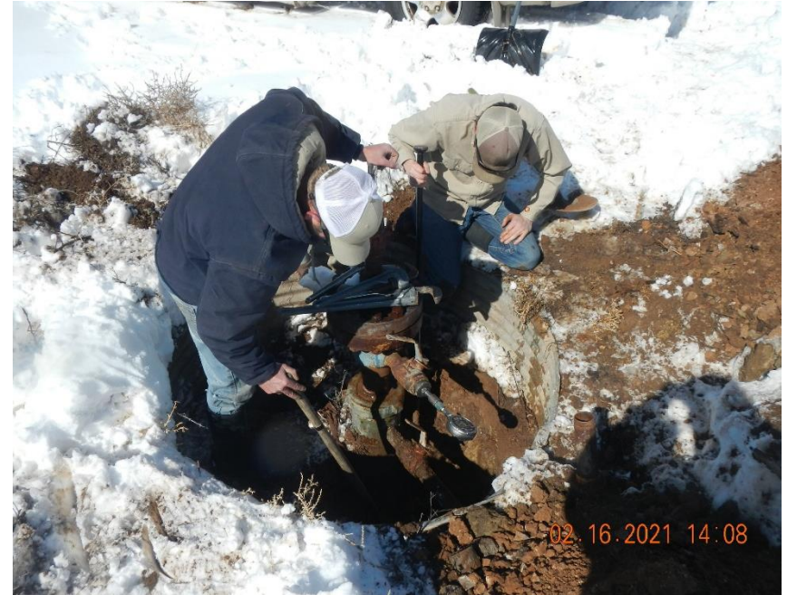
Cottonwood Consulting conducting Bradenhead testing.
