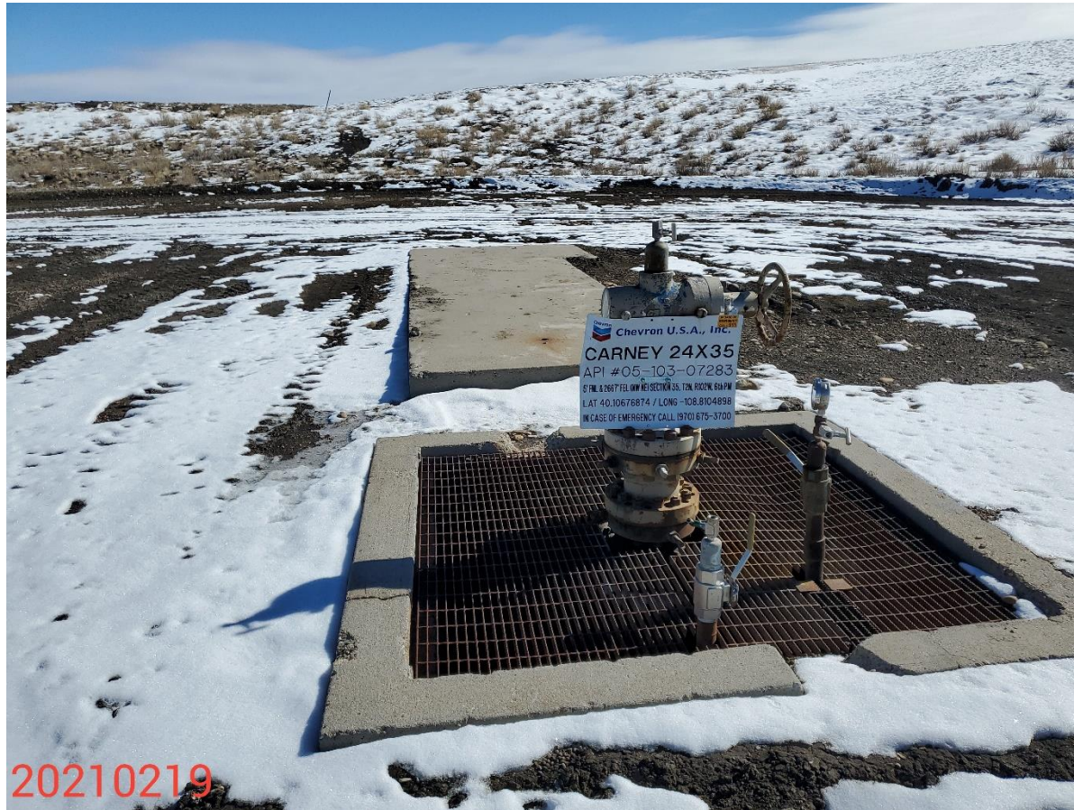
Photo 7: Photo of wellhead, signage and concrete based; Well shut-in
