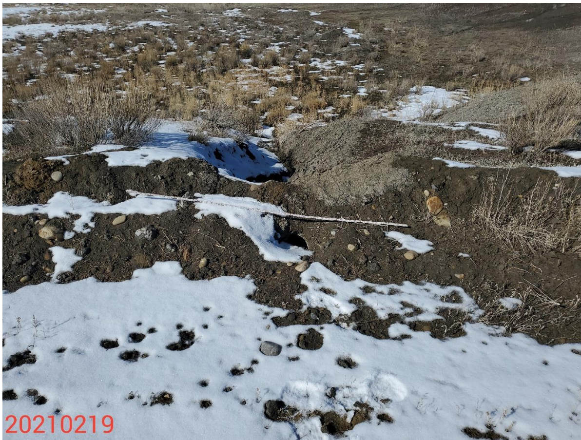
Photo 1: Photo taken from the northwest corner of the Location, facing west. Photo shows areas of the location where stormwater runoff has created a gully; stormwater and erosion control measures to protect/stabilize slopes and to allow for sediment laden-free stormwater discharge are missing, or insufficient. 6 foot measuring stick for reference.
