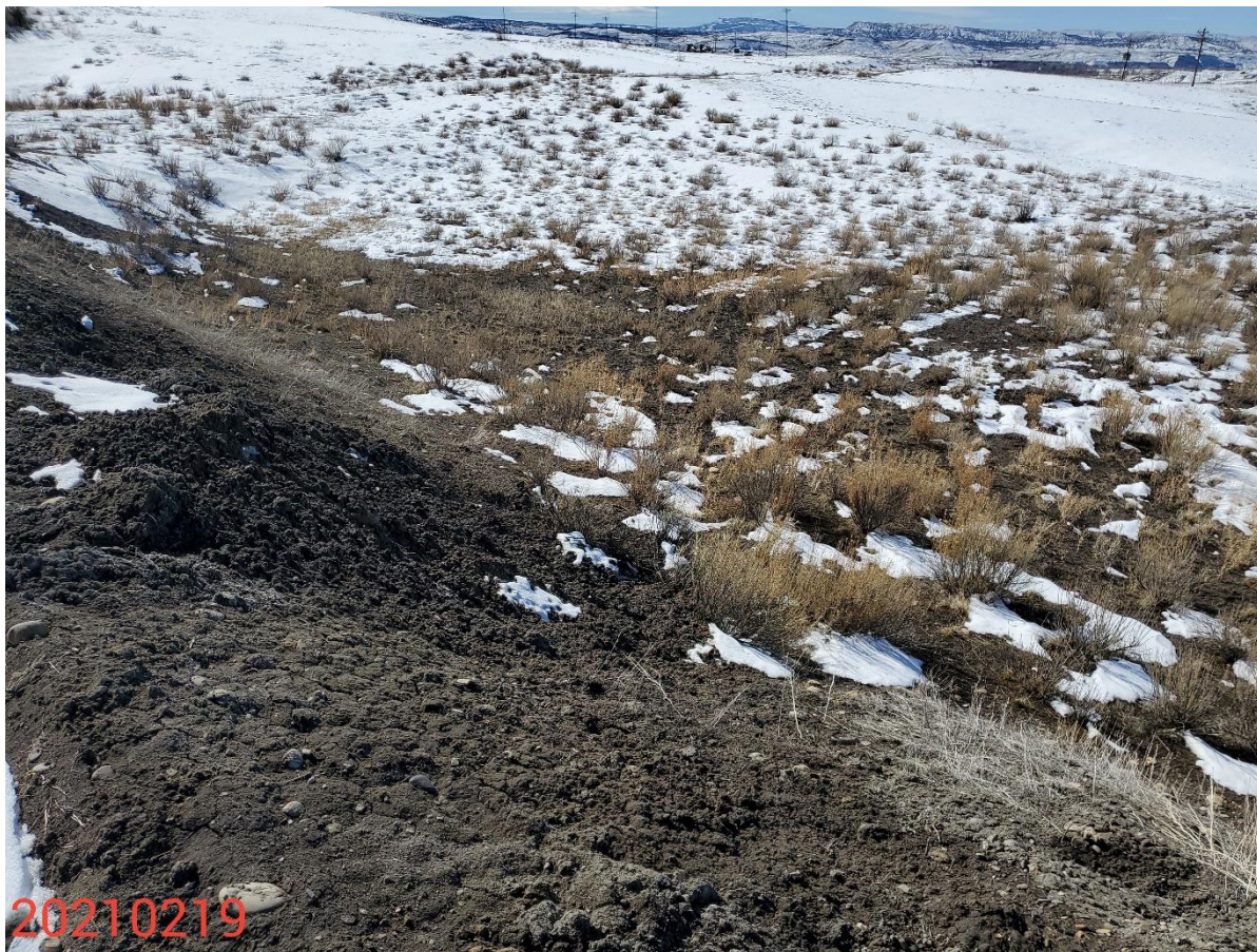
Photo 6: Photo taken from the west end of the Location, facing southwest. . Photo shows stormwater and erosion control measures to protect/stabilize slopes and to allow for sediment laden-free stormwater discharge are missing, or insufficient.
