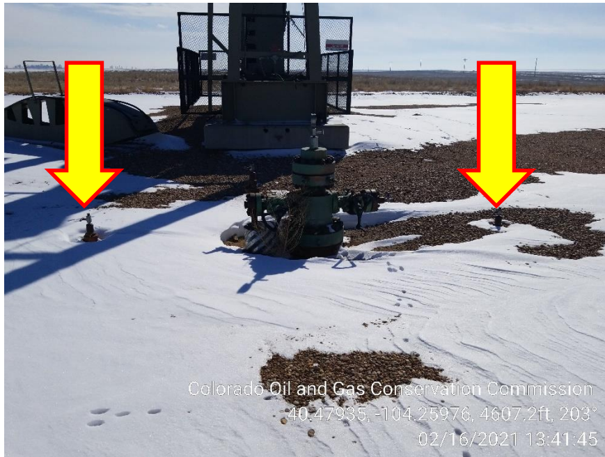
Photo 1 – Wellhead, Unmarked Risers
