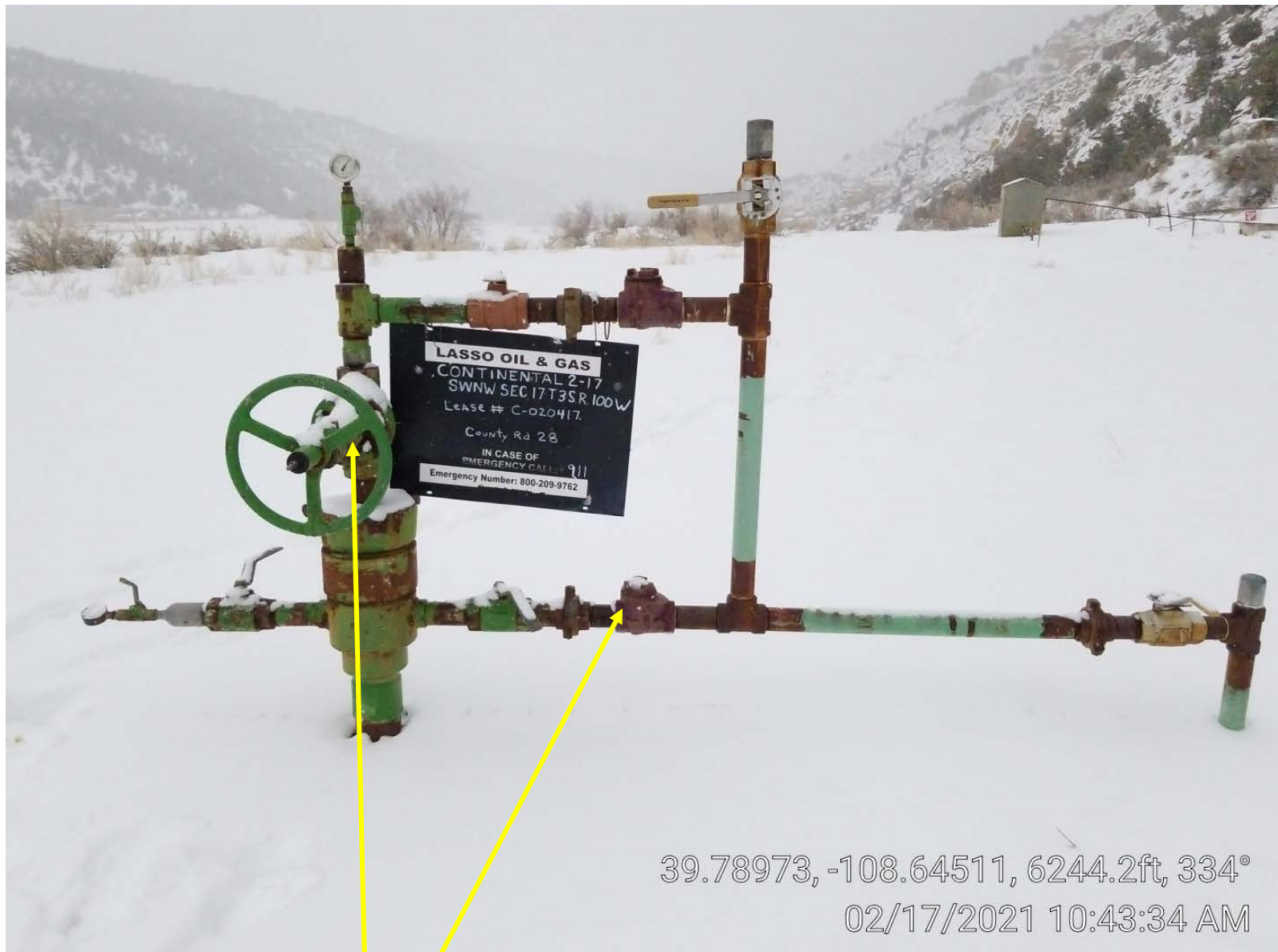
Photo 2. Well gas leaks.
