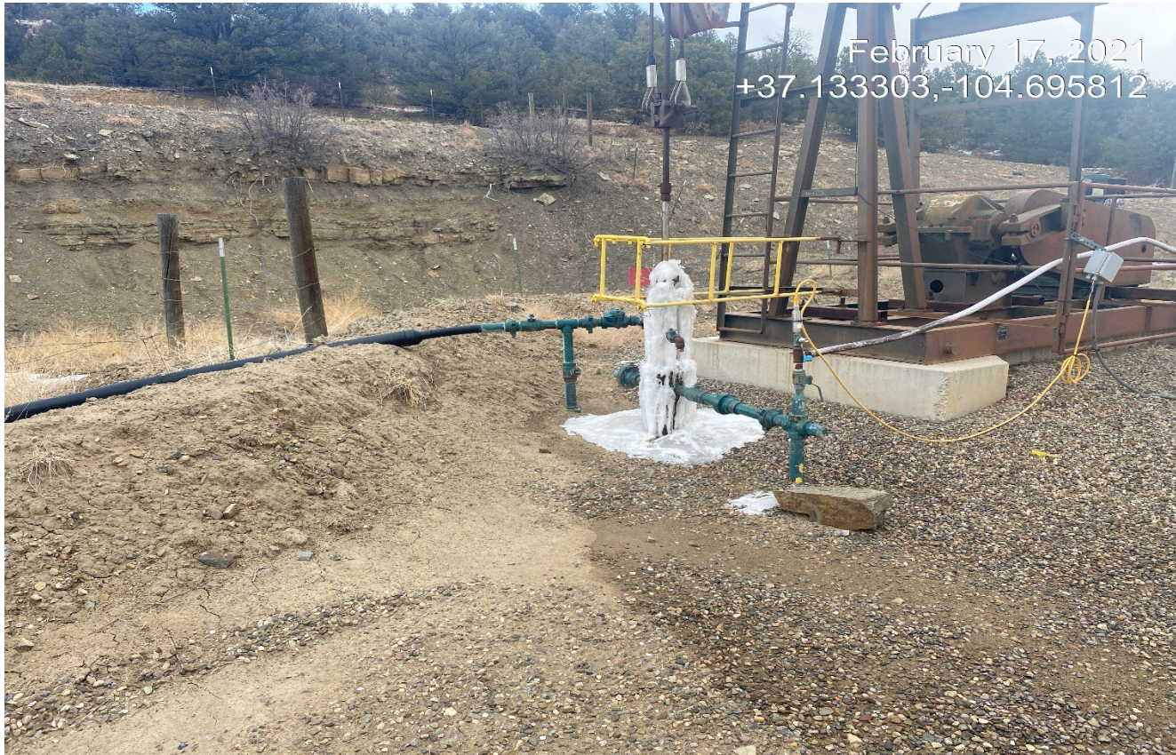
Photo 2. There is a leak at the wellhead which has turned to ice.
