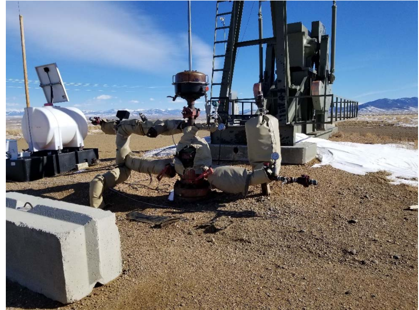
Photo 2. No bradenhead access apparent.
