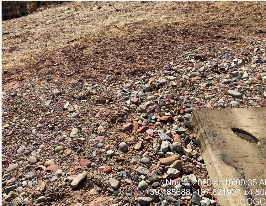
Sediment migration/erosion under combustor (photo from previous inspection)
