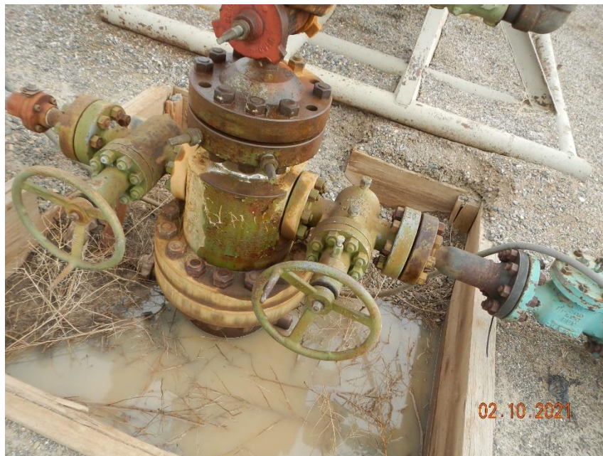
Stuffing box leak and over oiling rod oiler
