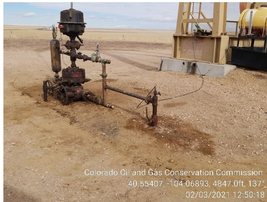
Photo 4 – Wellhead – Stained Soil
