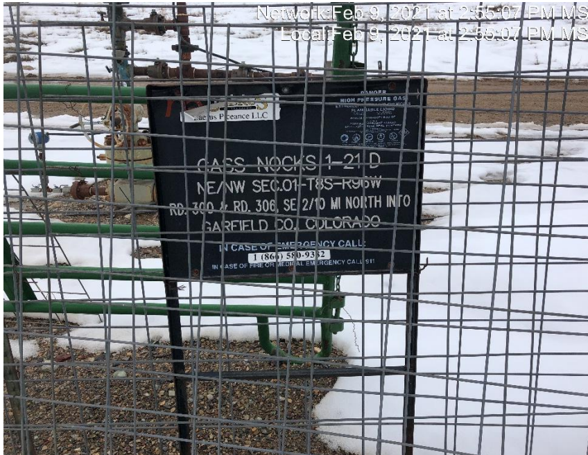
Photo #2864 All wellhead signs missing API number.
