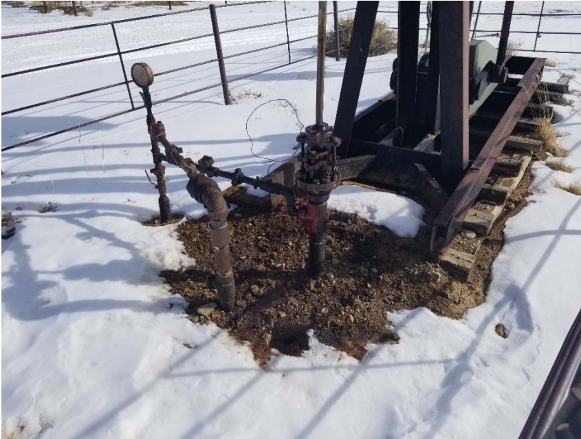
Photo 2. No bradenhead access apparent.
