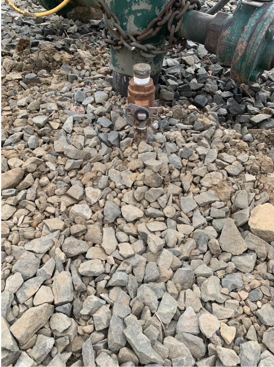
Braden head plumbed to surface
