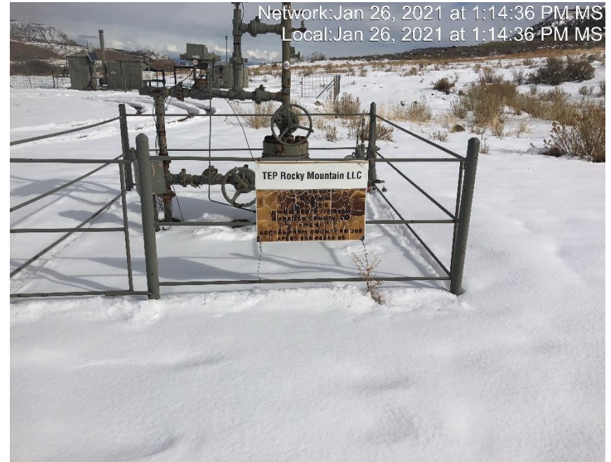
Photo #2712 Wellhead sign weathered and not legible.
