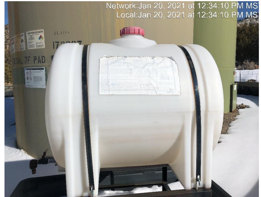
Photo #2668 Chemical tank label weathered and not legible.
