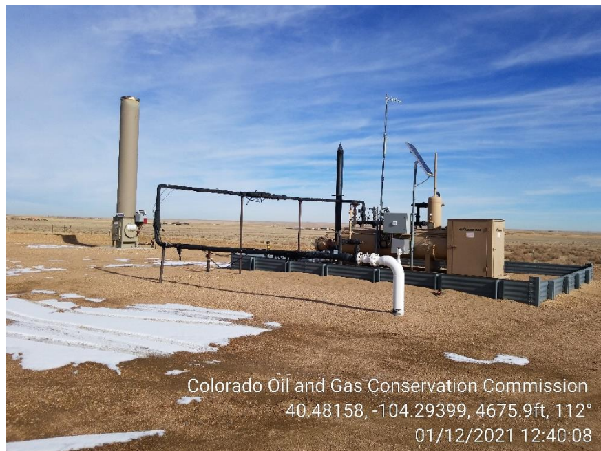
Photo 5 – Separator and ECD
