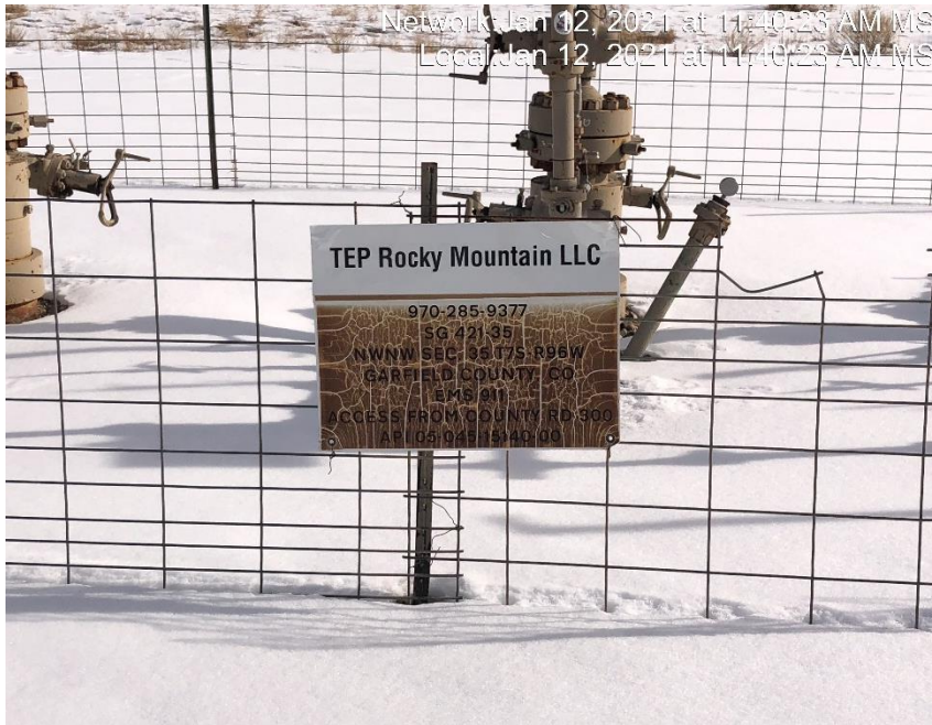
Photo #2612 Multiple wellhead signs weathered and not legible.
