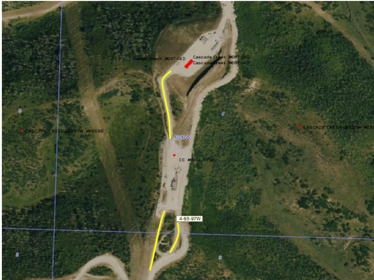
Photo 1: 2019 COGIS aerial image. Photo shows two parallel access roads leading to the CC 0604-1 Pad, and the Cascade Creek 697-04D. This does not comport with Rule 1002.e “surface disturbance minimization” requirements regarding access roads. Roads identified in yellow will require reclamation.
