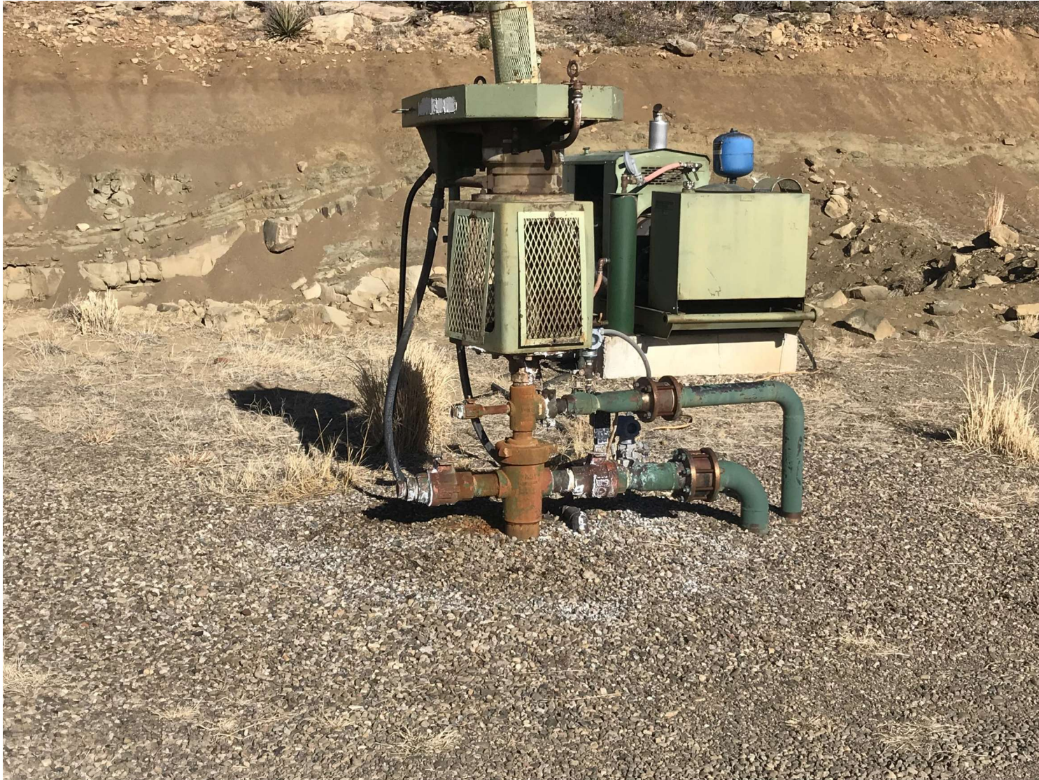
PHOTO 1: THE PACKINGS ON THE WELL HEAD WERE REPLACED TO ELIMINATE THE WATER LEAK.
