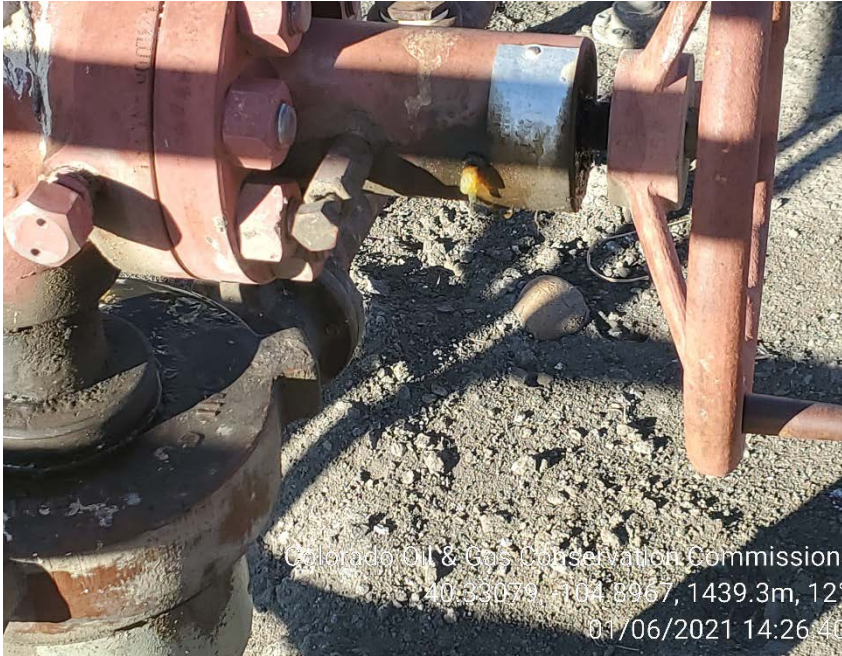
Master valve leak
