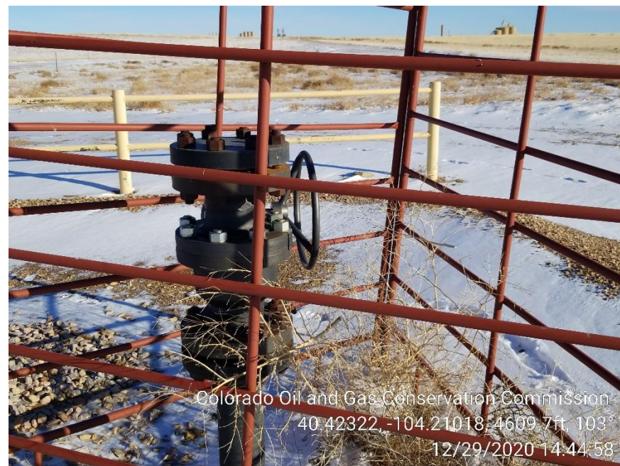
Photo 6 – Unmarked Riser
