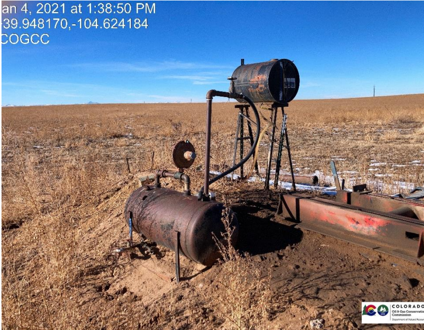
Pic 7 stained soil / no BMP under chemical tanks / weeds
