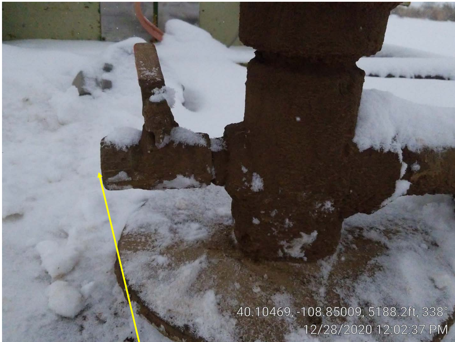
Photo 4. Well. Gas leak.
