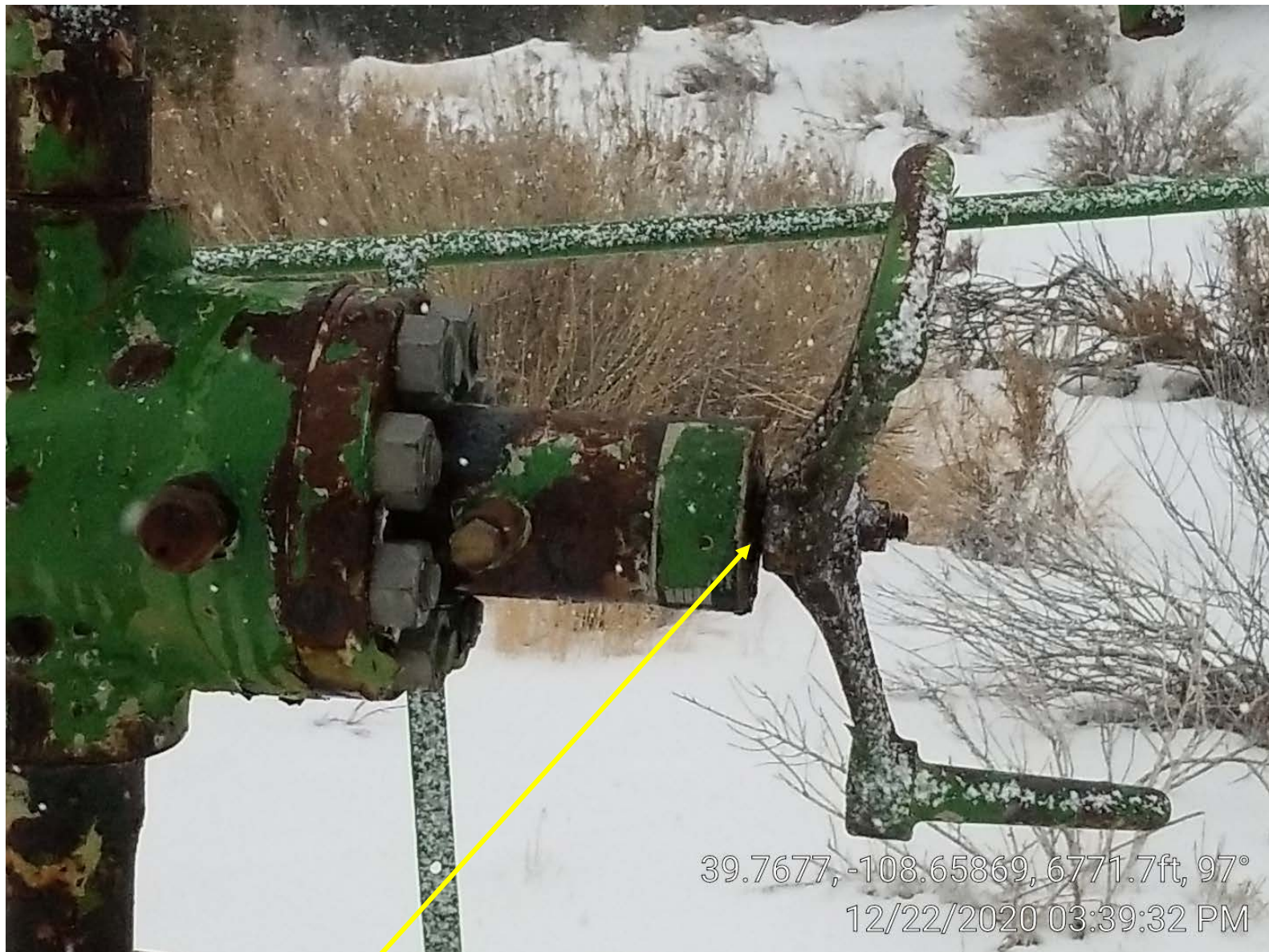
Photo 3. Gas leak.
