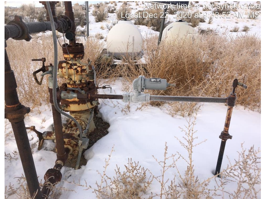
Photo #2519 supply gas valve to separator left opened.
