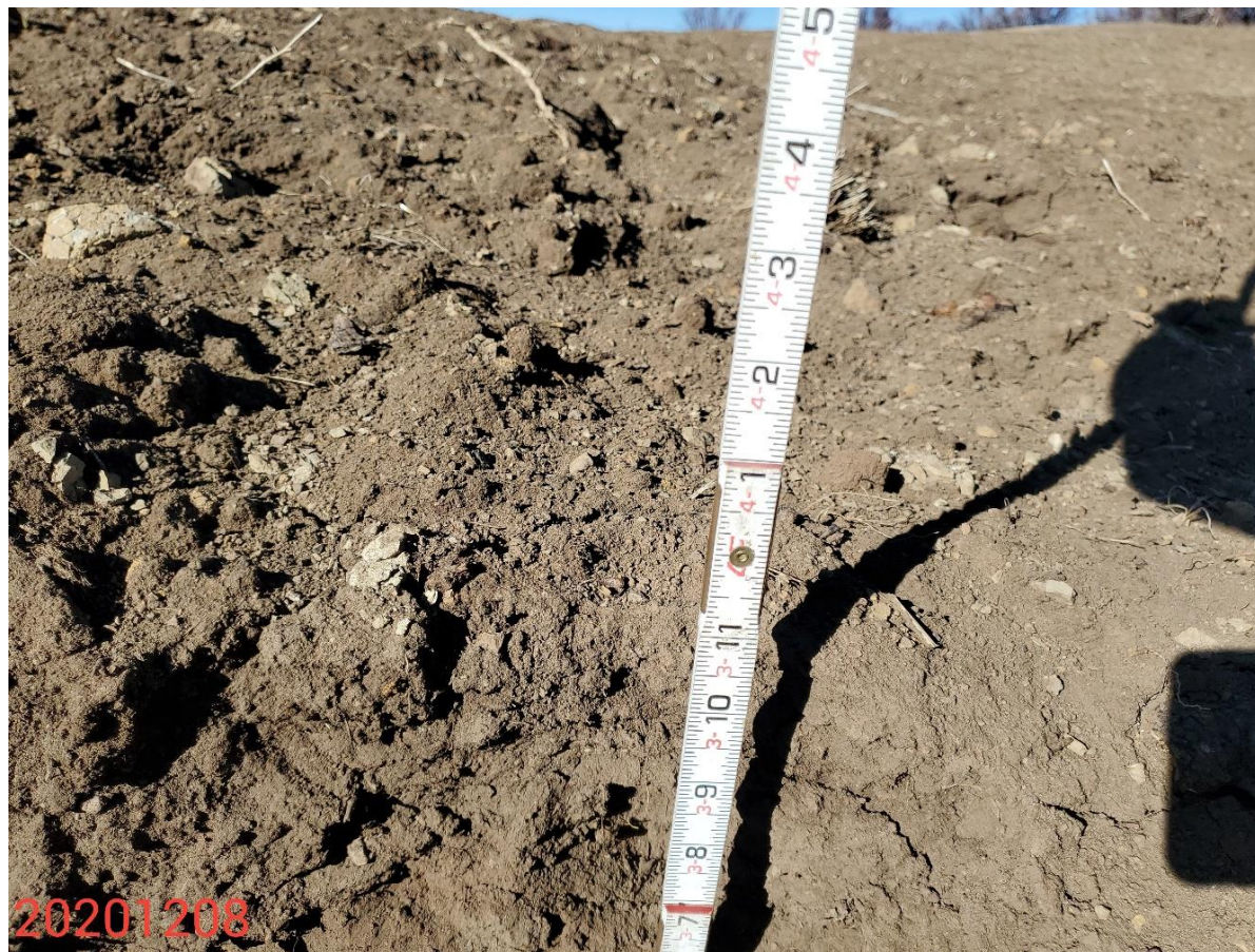
Photo 17: Continued from photo 15. Photo shows crack is ~4 feet deep; Soil/Slope stabilization concerns remain evident. 6 foot measuring stick for reference.
