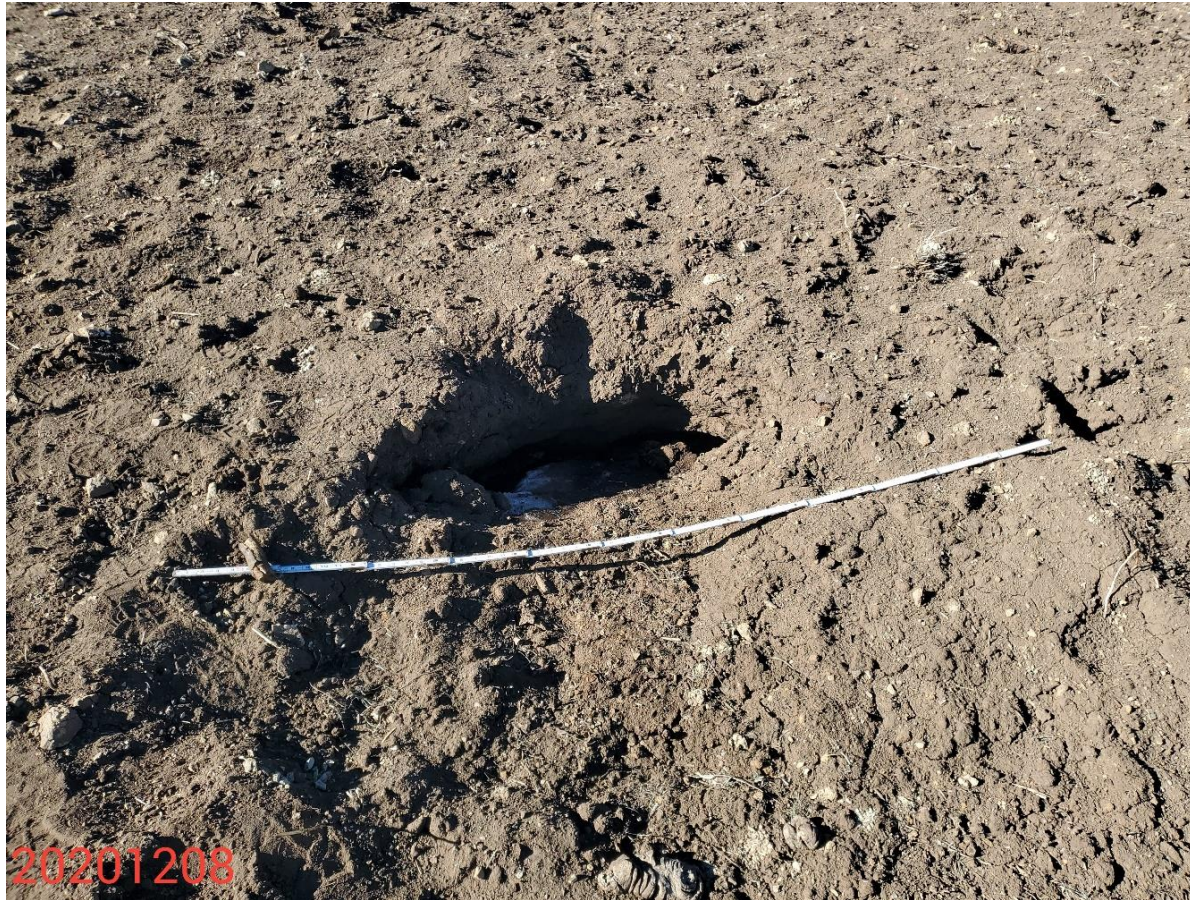
Photo 15: Photo taken from the southern interim areas of the Location. Photo shows cracking within the soils. Crack is currently ~3 feet wide, and 4 feet deep; Soil/Slope stabilization concerns remain evident. 6 foot measuring stick for reference.
