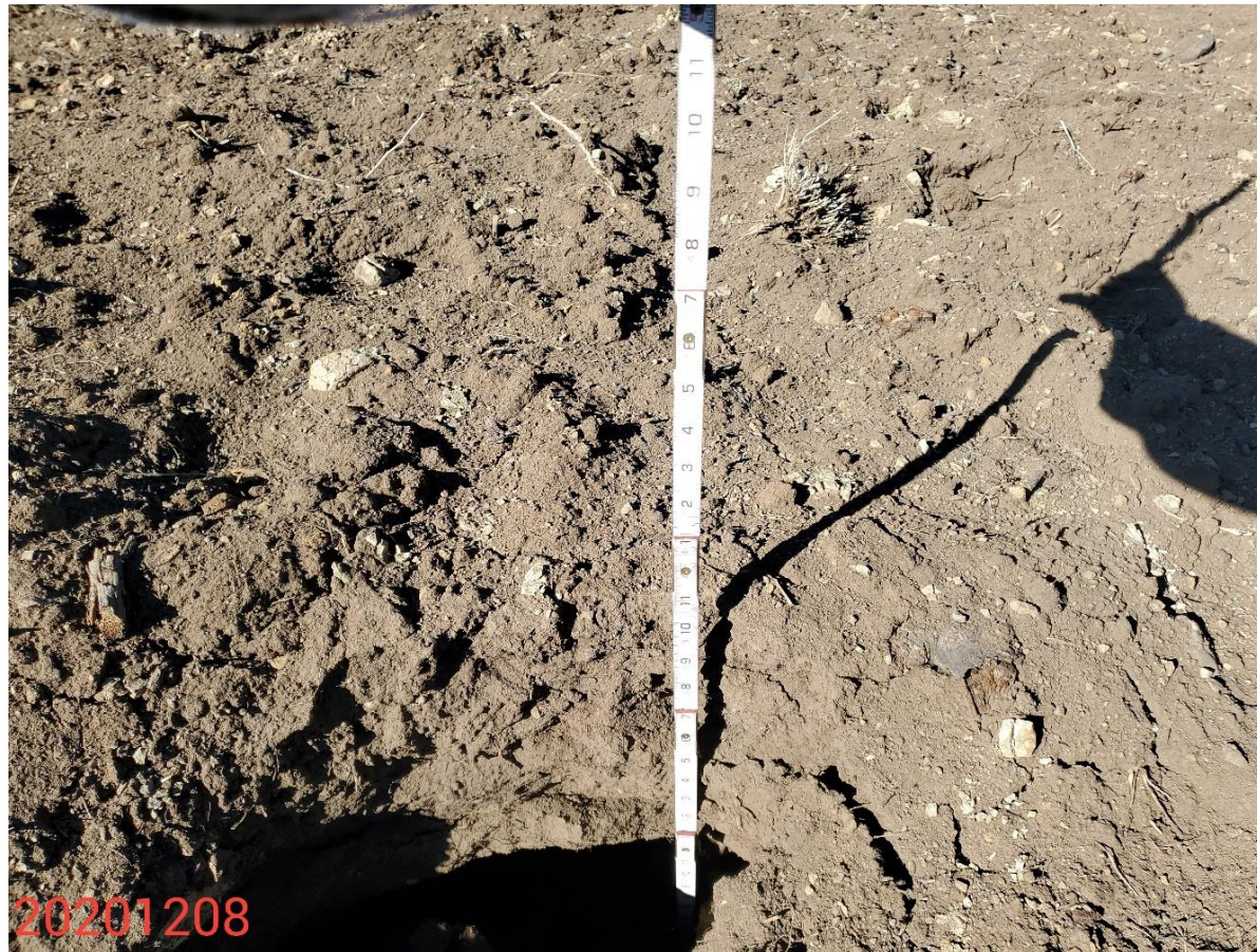
Photo 16: Continued from photo 15. Photo shows crack is ~4 feet deep; Soil/Slope stabilization concerns remain evident. 6 foot measuring stick for reference.
