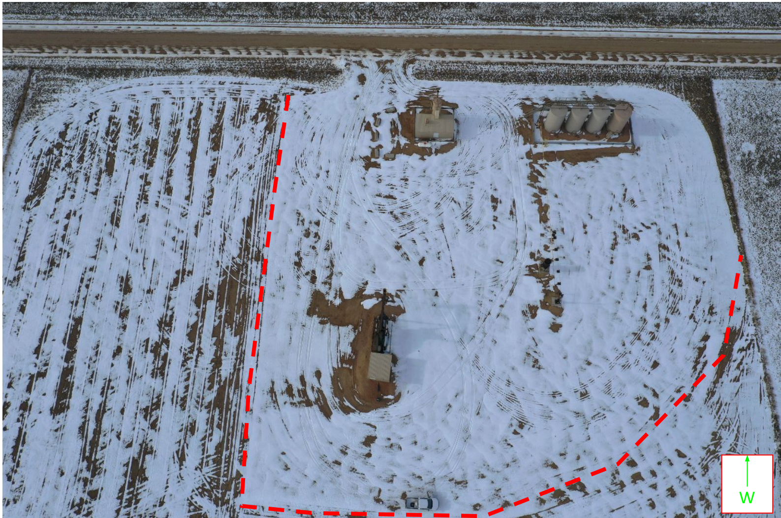
Photo 1. Drone aerial imagery taken on December 17, 2020. Photo illustrates the Operator has initiated interim reclamation activities to recontour and replace topsoil, but seeding does not appear to have been performed. Operator has not implemented any stormwater BMP's along the downslope of location but did leave the interim areas rough.
