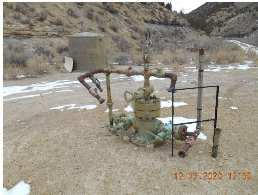
Wellhead with missing sign.
