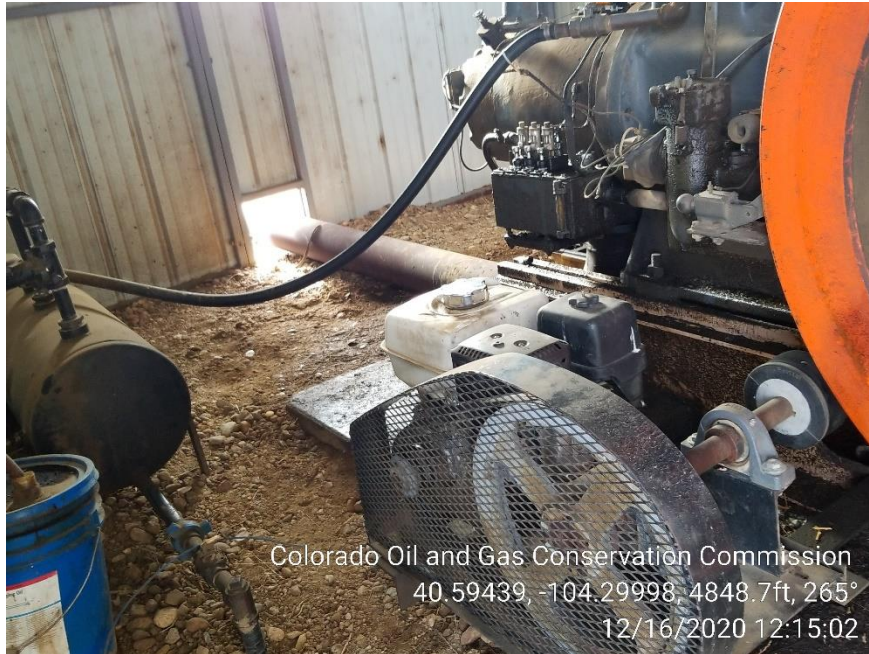
Photo 5 – Stained Soil at Gas Engine
