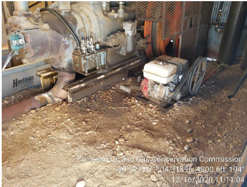
Photo 7 – Stained Soil at Gas Engine
