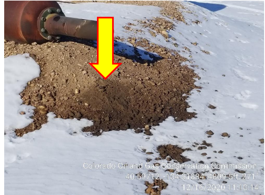
Photo 6 – Stained Soil at Engine Exhaust
