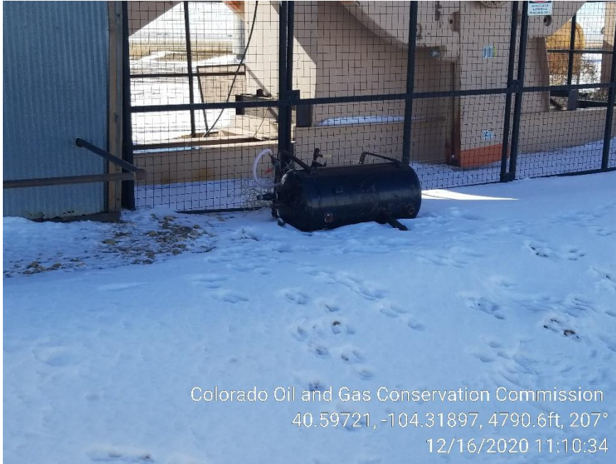
Photo 9 – Unused Supply Pot at Pumping Unit
