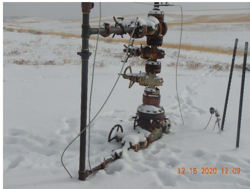
Photo 2. No bradenhead access apparent.
